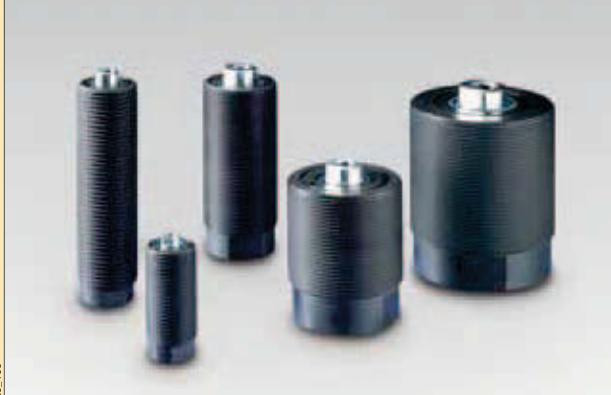
Threaded cylinders are designed for workpiece positioning, holding and ejecting applications where space is at a premium. Double-acting models are also suited to manufacturing applications, such as production punching.
