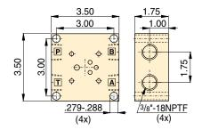
**Modular Valve Remote Mount Manifold**
