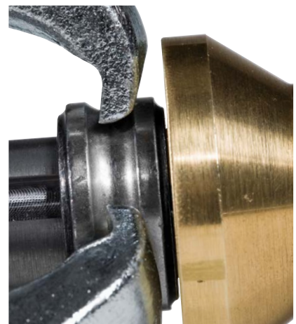
Lock on ball grooves and bearing races.
