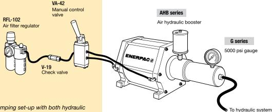
■ In an automated clamping set-up with both hydraulic and pneumatic components, AHB series boosters are used as a power source for the hydraulic system.
